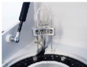
Washing Probe Independent 3 -step washing system.
