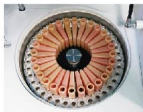
Reagent Tray Refrigerated tray with independent switch.
