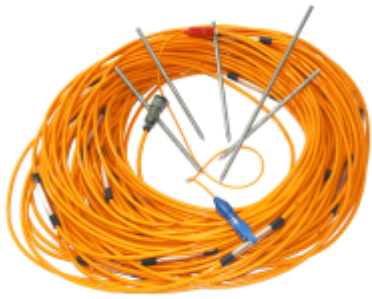
ERT cable systems
