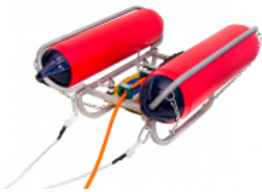
Electrodynamic source G-Boomer
