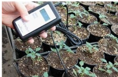
WaterScout SM 100 sensor shown with the FieldScout Soil Sensor Reader (Item 6466)
